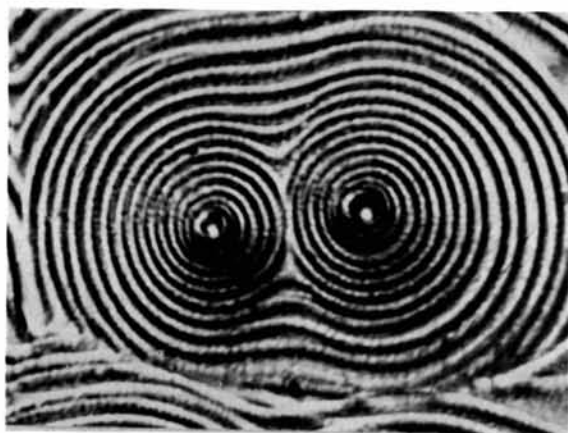
Fig. 4. Terraced pit showing a larger number of spiral turns ( \times 750 ).
