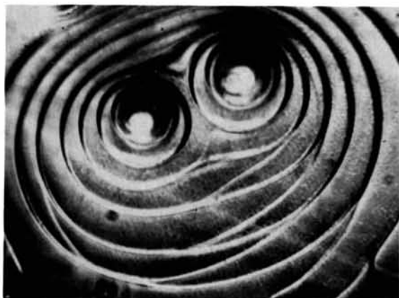
Fig. 5. Terraced pit with neighbouring loops connected by branches ( \times 750 ).
